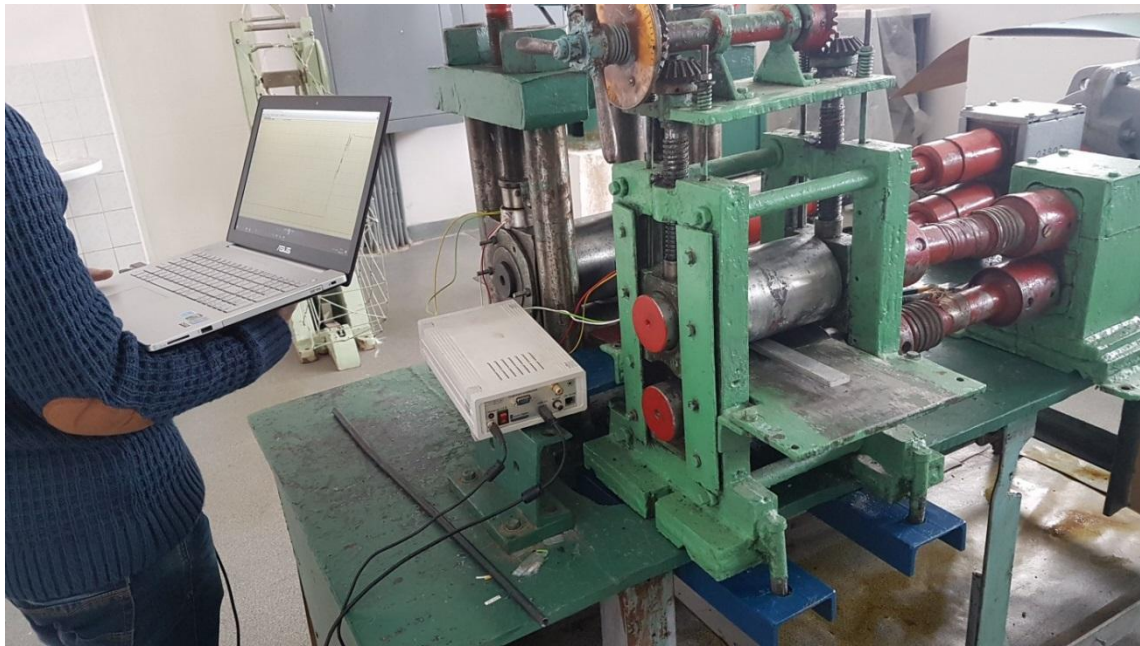
Fig. 4. Force measurement under “rolling – ECA-pressing” combined process”
