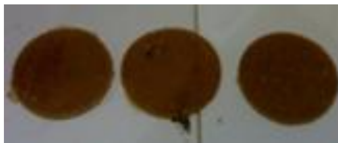
Fig. 3. Samples of composites reinforced with sawdust before compression test
