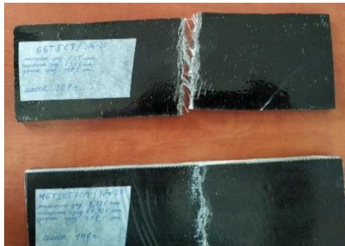
Fig. 5. Results of destruction of samples: (a) tensile; (b) bending
