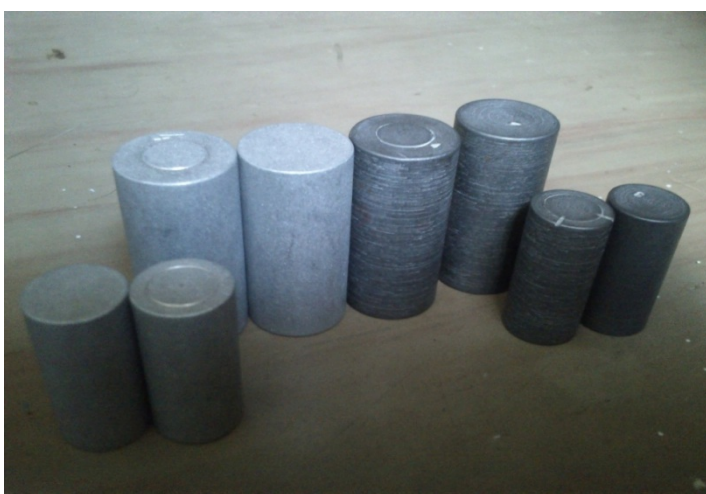
Fig. 3. Processed parts from aluminum D16 and steel 30GSA
