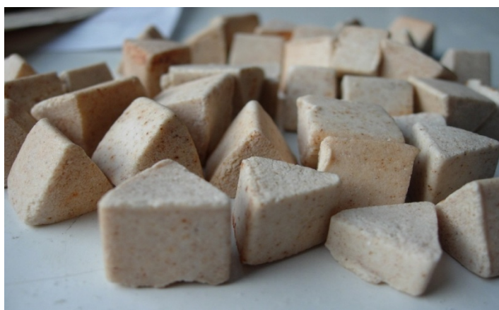
Fig. 2. Trihedral prisms, grain size 16
