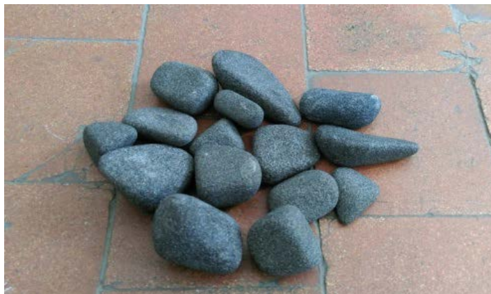
Fig. 1. Scrap of grinding wheels of 40×80, grain size 25
