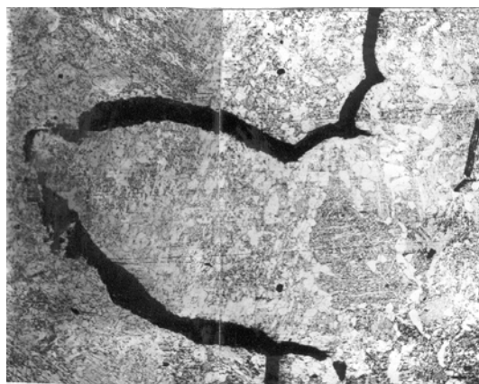
Fig. 1. TC nature in the electroslag weld joint of low-alloy steel, \times 100
