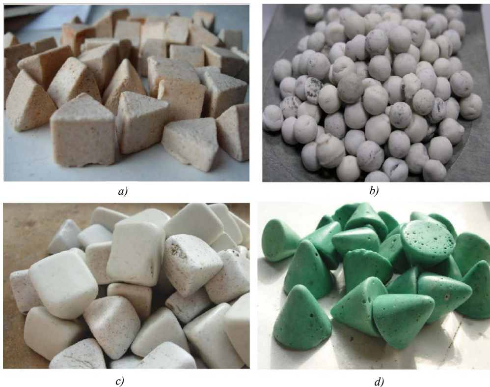
Fig. 5. Abrasive particles used in CRM: a) white prisms PT; b) porcelain balls; c) PT 25×25; d) white-green abrasive cone
