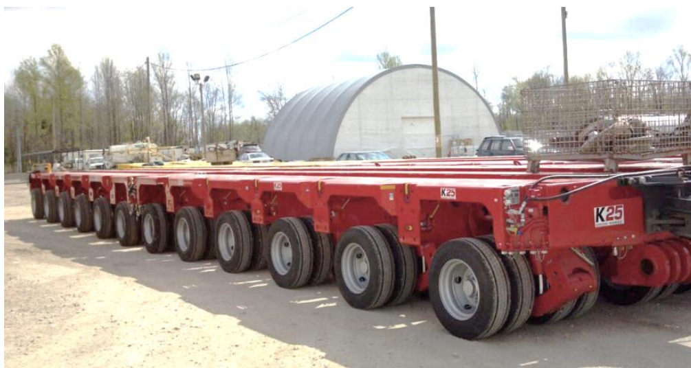
Fig. 2. Two connected 6-axis self-propelled InterCombi K25 modules from Kamag (Germany)
