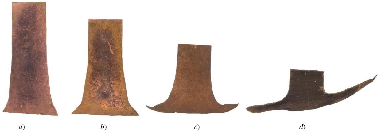
Fig. 1. Cross sections of copper samples after impact at different initial velocities: a — 162 m/s; b — 225 m/s; c — 316 m/s; d — 416 m
