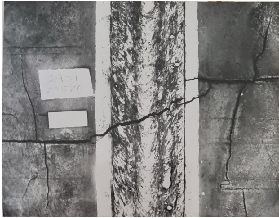
Fig. 5. Fracture nucleation and development pattern of the welded joint, whose interface zone was run between narrow beads (6th method):
