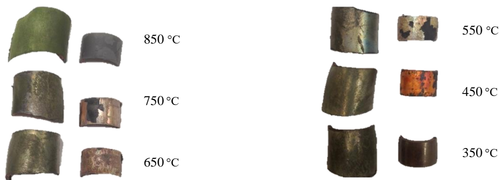
Fig. 7. Comparison of the outer surface of the samples after heating to the specified temperatures: on the left — coated samples, on the right — pure copper samples
