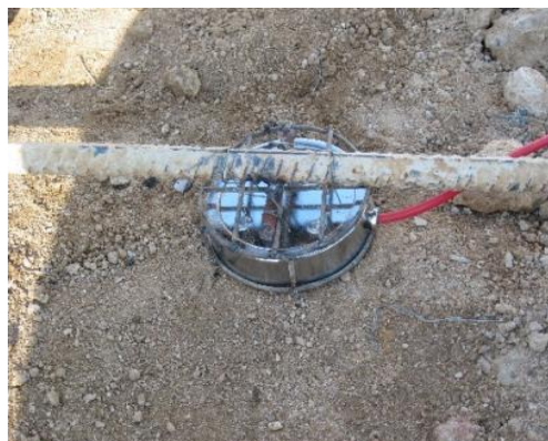
Fig. 3. Sensor for registering pressure in the soil and on the surface of the base layers [18]
