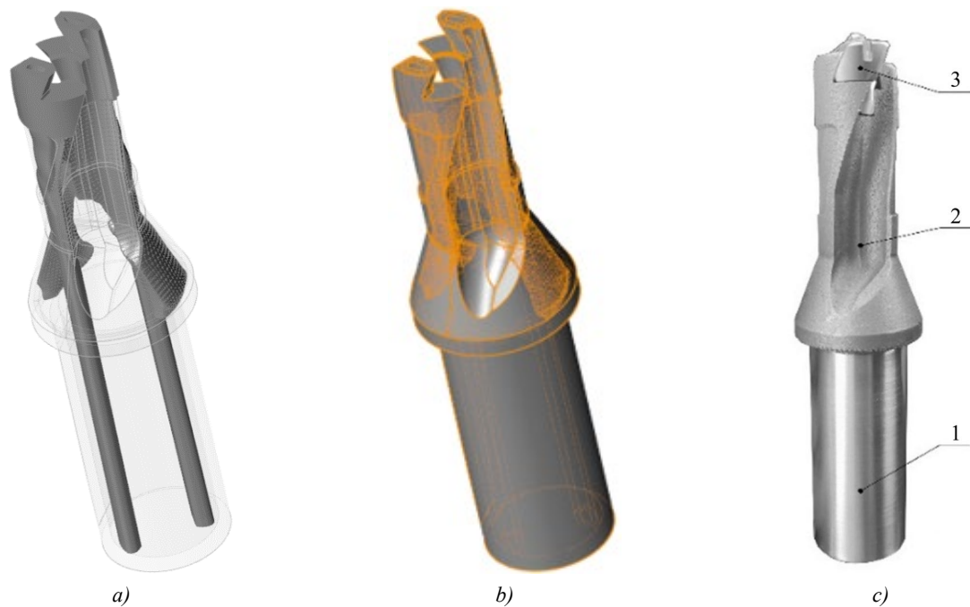
Fig. 1. Indexable drill: a — model of a topologically optimized part of a drill body with a setting head and curved cooling channels of the body; b — model of the TO drill body with a thin-walled shell forming the chip grooves and shank; c — physical sample of TO metal-composite indexable drill (cavity after TO is filled with MPCM), manufactured using SLM technology: 1 — machined metal-composite shank; 2 — chip grooves; 3 — cutting head of the indexable drill
