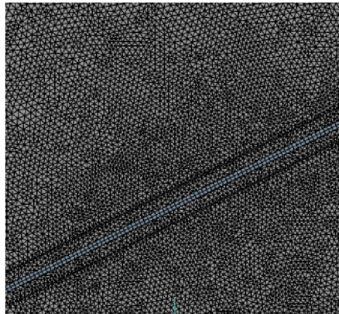
Fig. 3. Image of the constructed mesh on a model of a silicon wafer with a thermal memory element in a 100 μm wide dielectric pocket
