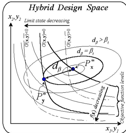
Fig. 2: Hybrid Design Space for normal distribution
