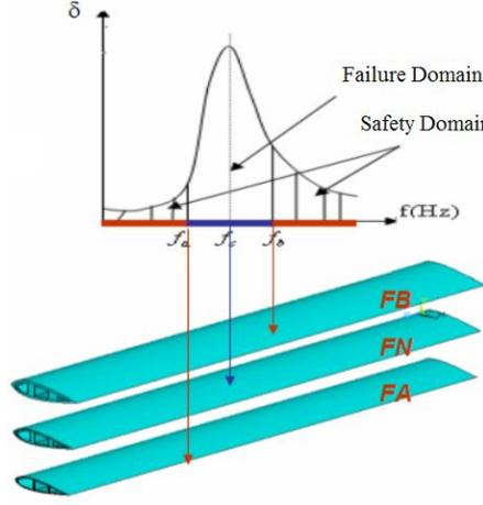
Fig. 5: Aircraft wing optimization models
