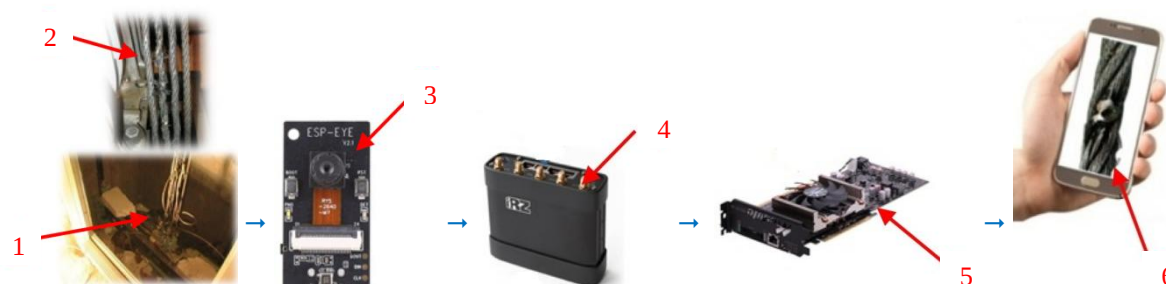
Fig. 2. PAC VIC functional diagram for detecting defects in steel ropes and balancing units based on computer vision and artificial intelligence technologies: 1 — balancing unit; 2 — rope defects; 3 — IP-camera; 4 — GSM-modem; 5 — neurocomputing device; 6 — image in a mobile device (the authors' figure)
