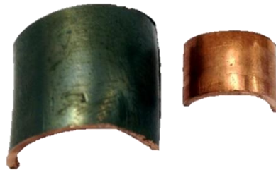
Fig. 6. Samples for the study of oxidation kinetics; external surfaces of reference samples of pure copper (right) and copper coated with Mo-Ni-Cr (left), prepared for experiments
