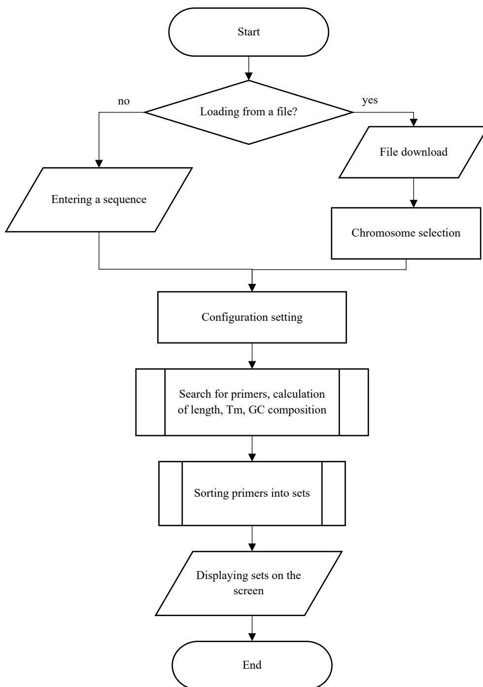
Fig. 3. Block diagram of the formation of primer sets for LAMP
