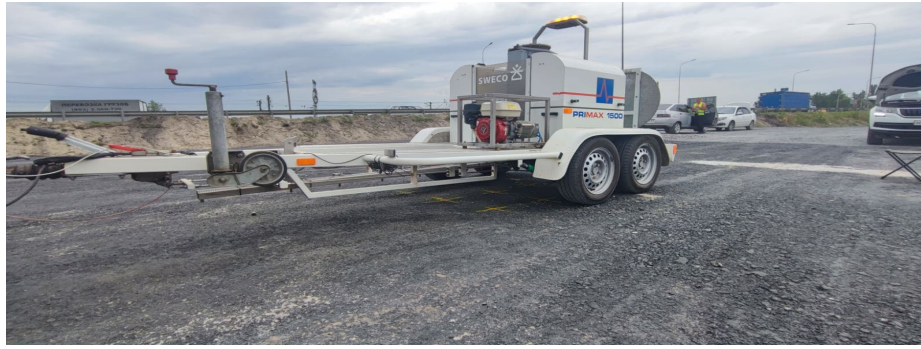
Fig. 4. FWD for recording vertical displacements on a layer of organomineral mixture
