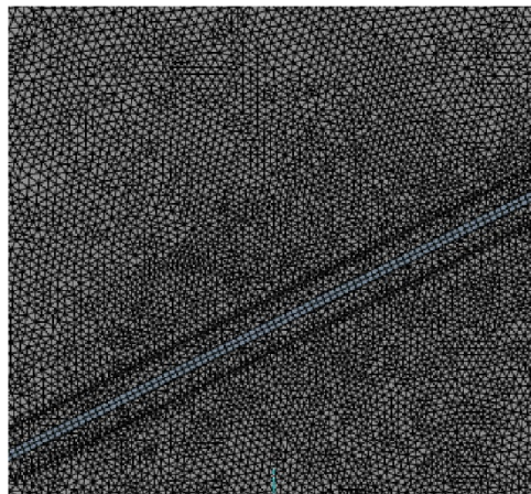
Fig. 3. Image of the constructed mesh on a model of a silicon wafer with a thermal memory element in a 100 μm wide dielectric pocket
